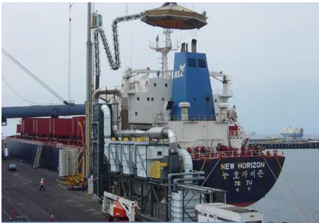
Land-based after-treatment technology demonstration, Tri-Mer
