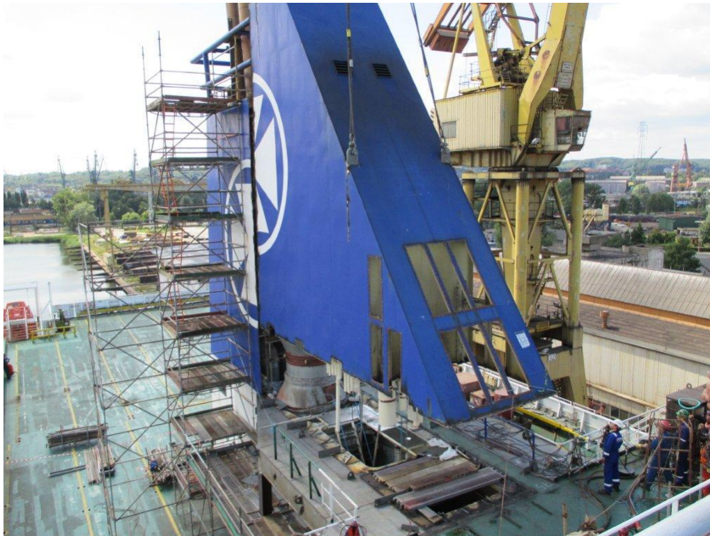
Figure 2.2: Preparations for installation of scrubber system, DFDS
