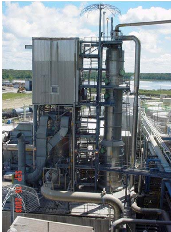
Figure 18 Chemrec 50 MW black liquor gasification plant at New Bern pulp mill
