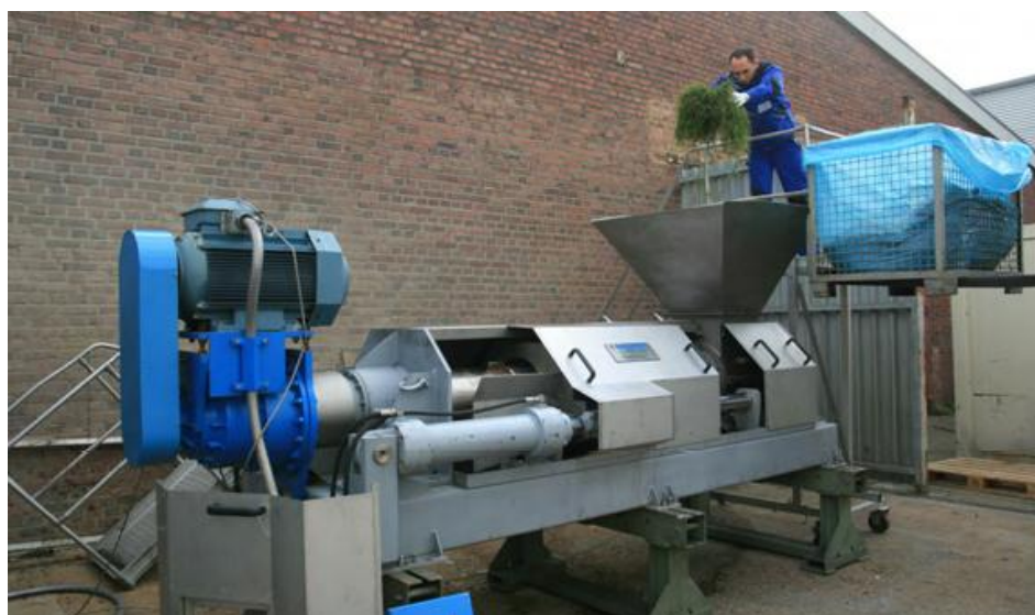
Figure 29 Mobile press for grass refining
