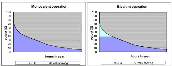
Figure 20 - Typical insertion of LTG into an annual load-time curve for a conventional district heating system
