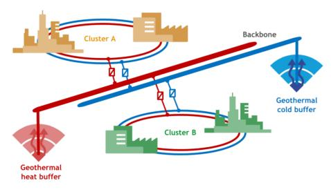
Figure 26 - Simplified schematic representation of the Minewater concept as implemented in Heerlen with geothermal buffering
