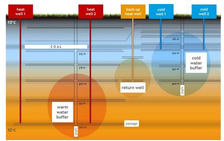
Figure 28 - Schematic picture of the subsurface Minewater system
