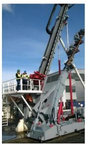
One innovation in the field of LTG is the combination of existing HDD (Horizontal Directional Drilling) technologies with oil/gas drilling technologies, permitting drilling to a maximum depth of around 1,250 m BGS using a relatively light, compact drilling platform.
