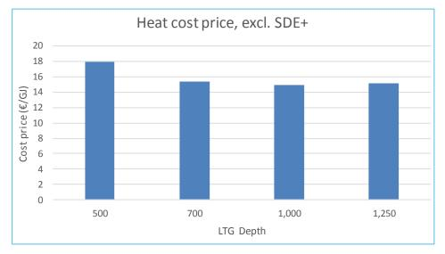
Figure 24 - Cost price of 50°C heat, including heat pump, excluding SDE+
