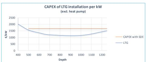
Figure 19 - CAPEX per kW as a function of depth
