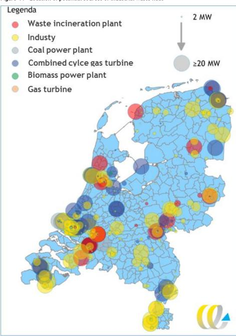
Figure 44 - Location of potential sources of industrial waste heat
