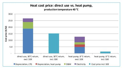
Figure 22 - Heat cost price: direct delivery vs. heat pump
