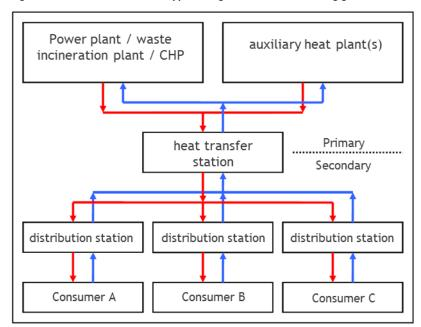
Figure 42 - Basic structure of a typical large-scale district heating grid
