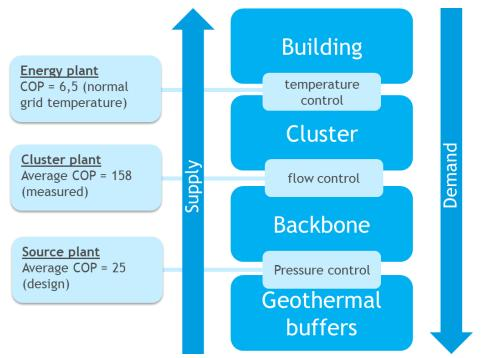
Figure 27 - Demand-driven plant and equipment in the Minewater system applied in Heerlen
