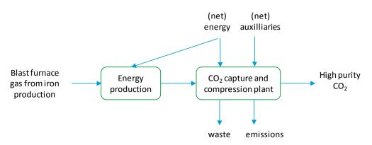
Figure 4 - Schematic representation of carbon capture from blast furnace gas from iron production
