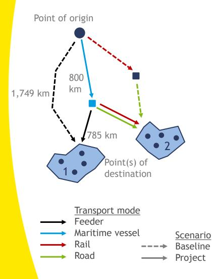
Calculation based on links (from point of origin to point of destination) using relevant routes & modes
