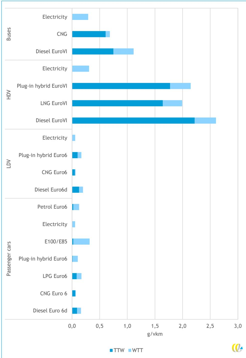
Figure 2 - Emission factors of PM<sub>10</sub> (tank-to-wheel and well-to-tank) for different vehicle technologies
