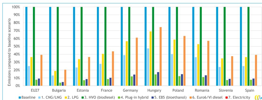
Figure 12 - Residual NO<sub>x</sub> emission (TTW) per scenario compared to baseline of heavy goods vehicles in 2030
