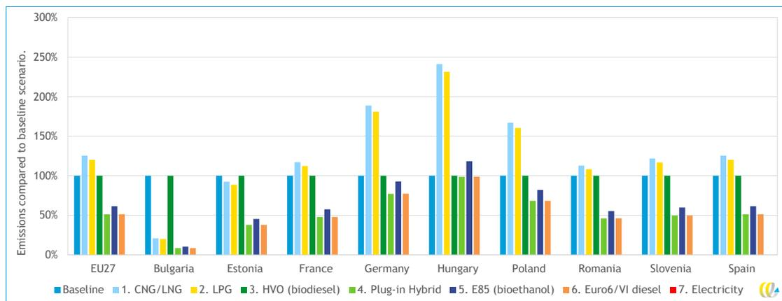
**Figure 14 - Relative reduction per scenario in PM<sub>10</sub> emission (TTW) of HGV's in 2030**
